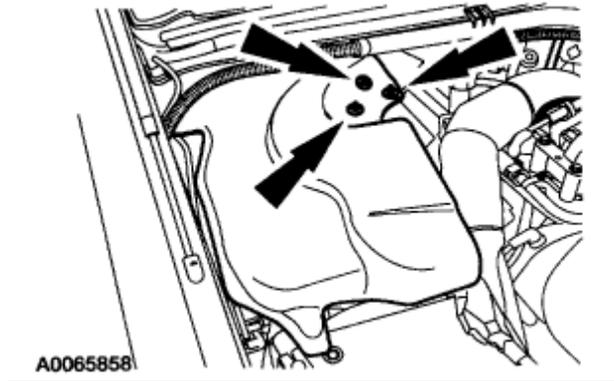
2. Remove the retainers and the insulator (6.0L diesel).
