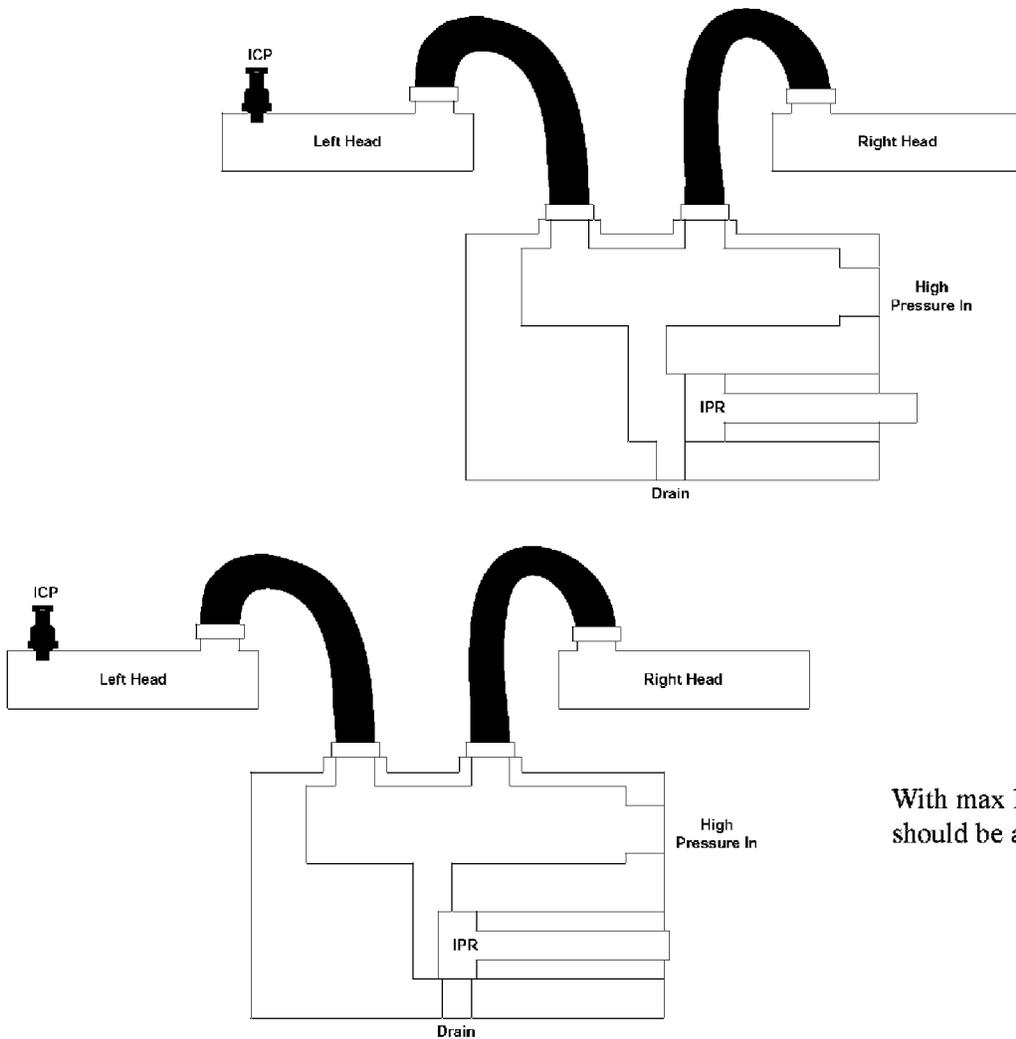
The IPR acts to increase ICP by restricting the path to drain.
