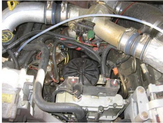
Find the drain valve behind the filter housing and move the yellow lever to the right to drain the fuel from the filter housing.
