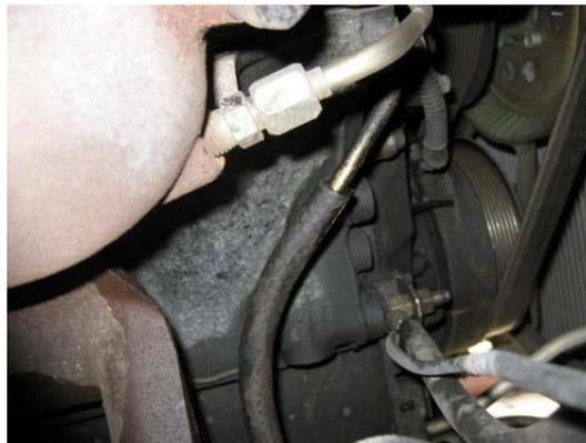
Remove the cover that goes over the fuel filter housing (this is a good time to replace the filter).....
