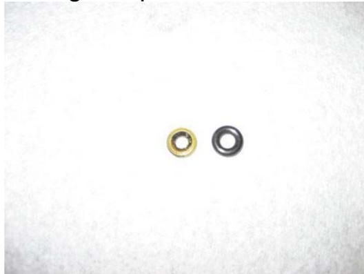
I used a pick tool to remove the old o-rings. To install the new ones just push them into place and they will fit like a glove
